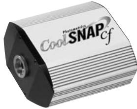
The CoolSNAP<sub>cf</sub> Monochrome camera from Photometrics® incorporates low-noise electronics and moderate CCD cooling to achieve good low-light sensitivity. A megapixel sensor with small, square elements ensures that each image shows extraordinary detail. This feature, along with a high-speed digitizer, shutterless operation, and an interline-transfer CCD, makes the CoolSNAP<sub>cf</sub> Monochrome camera ideal for high-resolution microscopy and inspection applications.
