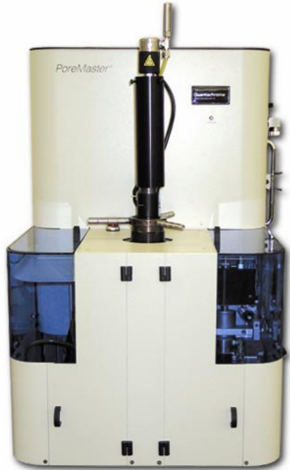
The programmable PoreMaster® mercury intrusion porosimeter.
