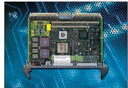
Dual gigabit Ethernet interfaces and four asynchronous RS232/422/485 lines provide a range of high-speed networking and connection
