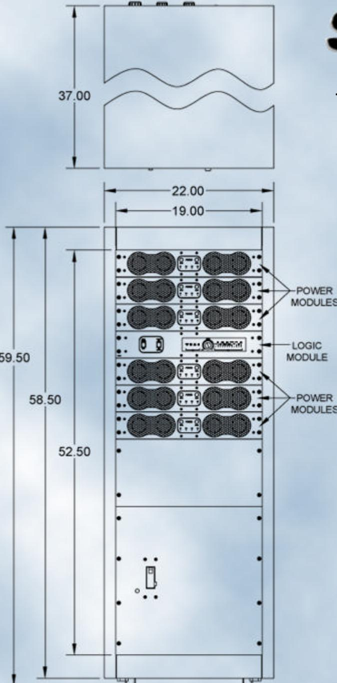
The DSA 36/48 Power Amplifier is designed to accept up to (6) six output modules of either the DPM-6 or DPM-8 configurations.
